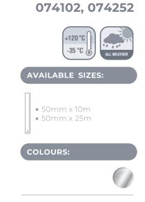
General purpose aluminium tape with high tensile strength aluminum foil backing, combined with a cold weather acrylic adhesive, protected by an easy-release silicone release paper.
