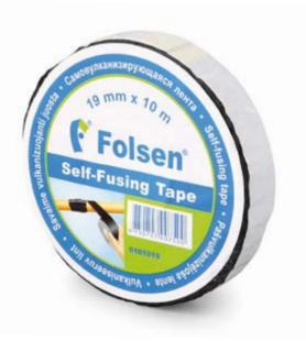
Very flexible insulating tape made of special PIB rubber. The tape has excellent electrical and physical properties, which allow it to "sinter" fast into homogeneous mass without the influence of heat. Good for protecting hoses, plastic and metal tubes as well as other automobile, industrial and household appliances against corrosion.
