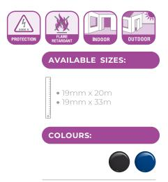
This tape is based on a 0.10 mm soft PVC film, coated with an aggressive rubber- resin adhesive with flame retardancy and good aging characteristics. Excellent conformability and high elongation at break.
