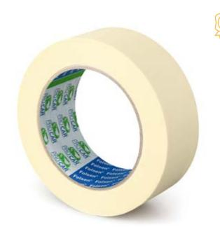
Crepe paper masking tape with high performance, specific for automotive sector during collision repairs and painting processes with drying cycles at high temperatures up to 110 °C (for 30 min). It combines controlled unwinding, easy tear and conformability. Well performing in overlapping the tape, with masking paper and masking film, it provides excellent paint edges, clean and safe removal without residues and breaking.
