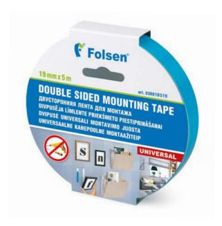
This tape of 1.1 mm thick PE foam is coated with modified acrylic adhesive on both sides with blue protective liner. The tape ensures high adhesion, resistance to movement and is adapted to different weather conditions.
