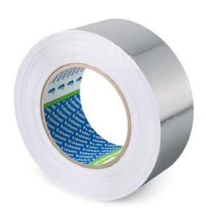
Aluminium tape with acrylic adhesive, based on solvent. High breakage strength aluminium foil backing. This tape is low temperature resistant and it works fine at high temperatures - up to 150°C. Used in the HVAC industry for joining and sealing Foil-Scrim Facing; for joining and sealing flexible air duct seams and connections.
