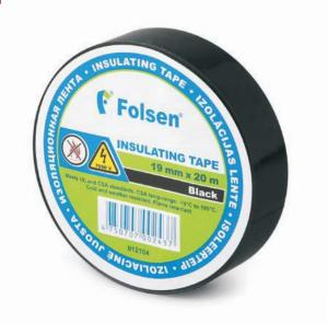
Based on PVC film, this insulating, flame retardant tape is strong and highly durable and can be stretched without breaking. Its rubber adhesive has good ageing characteristics. This tape is meant for use in electrical insulation, bundling, coding identification and marking on joints and splices in wires, pipe and cable.
