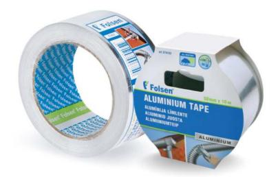
General purpose aluminium tape with high tensile strength aluminium foil backing, combined with a cold weather acrylic adhesive, protected by an easy-release silicone paper. Cold weather acrylic adhesive offers good sealing and bonding on Foil-Scrim-Kraft Facing joints and seams in a HVAC ductwork application.
