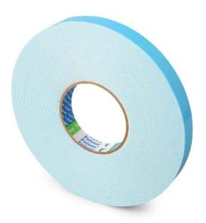
This tape of 1.1 mm thick PE foam is coated with modified acrylic adhesive on both sides with blue protective liner. The tape ensures high adhesion, resistance to movement and is adapted to different weather conditions.
